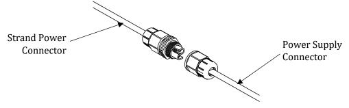
14. Connect the power lead wire to the appropriate 12V DC power supply.
