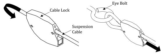
7. You can tighten the suspension cable using a catenary tensioning tool or loosen the cable using a cable release key on the cable lock.
