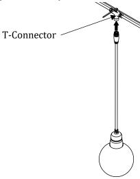
13. Connect the strand power connector to the power supply connector.
